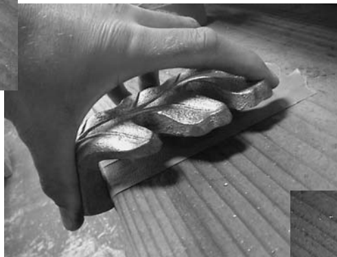
Push part flush to edge, then depress the mark so that the "marking studs" make an impression on the tape.
